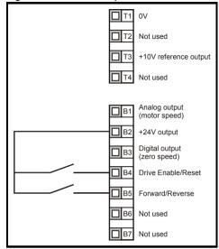
Figure 7-2 Minimum required control terminal connections
