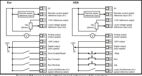
Terminal B7 open: Local voltage speed reference (A2) selected Terminal B7 closed: Remote current speed reference (A1) selected
