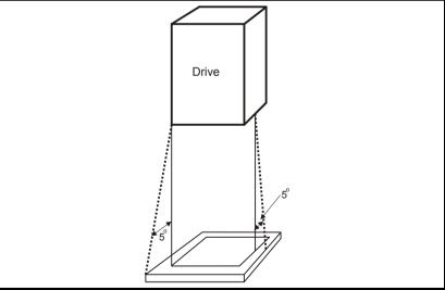
The bottom, including the part of the side considered to be part of the bottom, must be designed to prevent escape of burning material - either by having no openings or by having a baffle construction. This means that openings for cables etc. must be sealed with materials meeting the 5VB requirement, or else have a baffle above. See Figure 3-2 for acceptable baffle construction. This does not apply for mounting in an enclosed electrical operating area (restricted access) with concrete floor.
