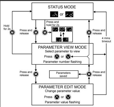
When in Status mode, pressing and holding the (1) MODE key for 2 seconds will change the display from displaying a speed indication to displaying load indication and vice versa.
