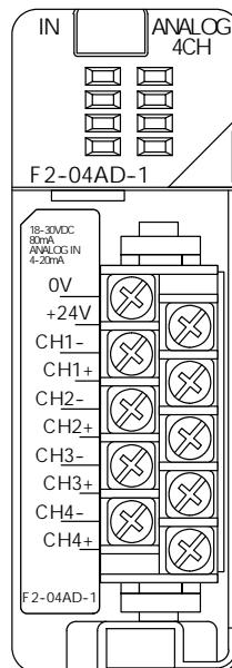
More than one external power supply can be used provided all the power supply commons are connected. A Series 217, 0.032A, fast-acting fuse is recommended for 4-20 mA current loops. If the power supply common of an external power supply is not connected to 0VDC on the module, then the output of the external transmitter must be isolated. To avoid "ground loop" errors, recommended 4-20 mA transmitter types are:
