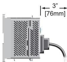
**NOTE:** Add 3 inches (76 mm) to mounting depth when using ZIPLink cable ZL-CBL40.
